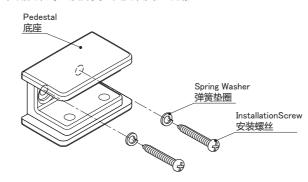
②Fit the body to the pedestal and secure it with the fixing screws and spring washers provided
